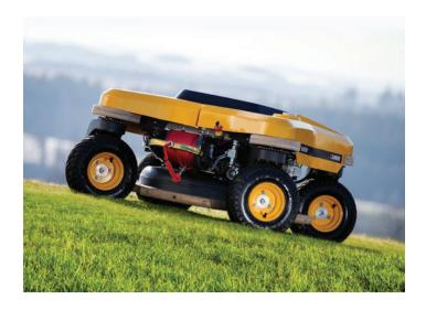
The SPIDER CROSS LINER is sure to impress with its innovative and compact design. This well-equipped commercial lawn mower features a terrain-copying platform, integrated stabilizing winch, and skid-steering option.
